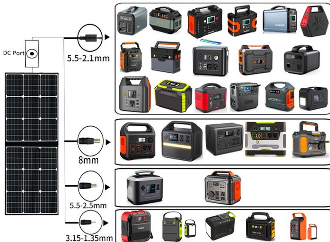
Different sizes of DC connectors for most solar generators
