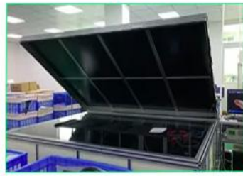
EL testing for foldable solar panel
